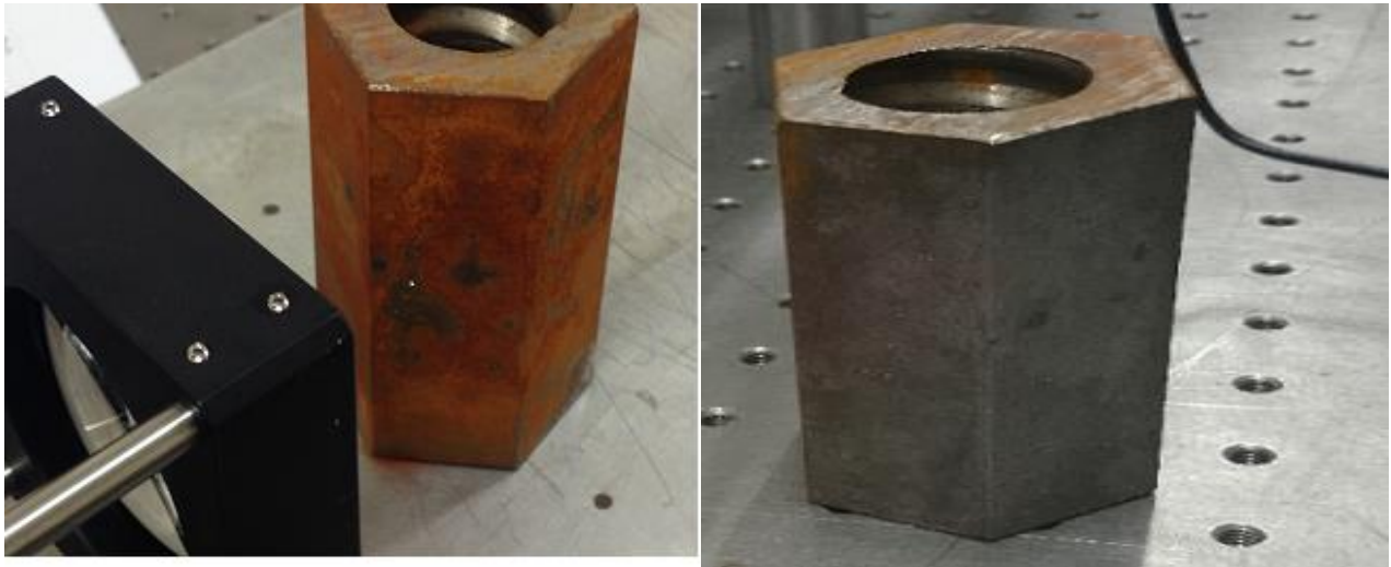
Fig.1 Mild Steel sample showing rust layer and regular surface sections
